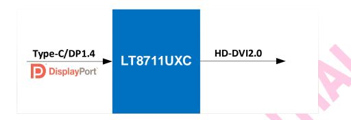
Figure 3.1 Application Diagram
